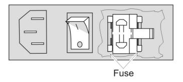
Figure 5-1: AC Fuse Replacement
